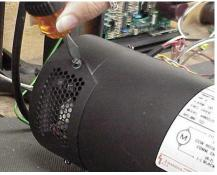
Locate the brush and the clip holding it in place. On one side of the motor, the clip will be under the brush, and on the other side it will be on top of the brush.
